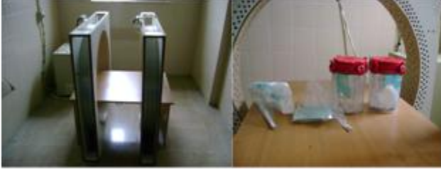
Figure 1. The cylindrical solenoid electromagnetic field apparatus used for exposure of H. pylori NCTC 11637 to EMF (50 Hz of frequency and 3.0 mT of intensity). The bacterial suspensions of H. pylori contained in anaerobic jar and Cook roasting bag transparent to the EMF was located on the middle part of the magnetic field inside the coil system.
